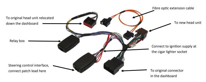
The original head unit needs to remain connected to the audio system in order to retain the use of the navigation and vehicle information screen.
