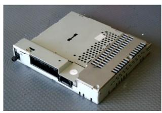
Refit the circuit board into the tray and refit the heat sink and lid.
