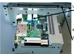
Undo the screws to remove the top lid.
