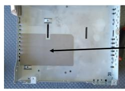
Undo the screws below the circuit board. Make sure the insulating sheet stays in place.
