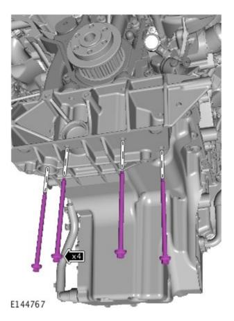
Install the oil pump lower retaining bolts.
