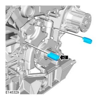
Remove the timing belt cover sealing strips.
