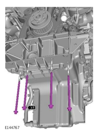
Remove the oil pump lower retaining bolts.
