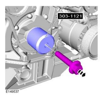
Remove and discard the crankshaft pulley retaining bolt.
