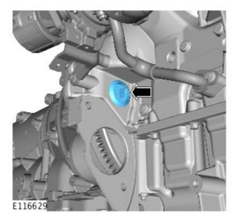
5. Rotate the crankshaft clockwise to align the crankshaft alignment hole in the flywheel or flexplate with the block aperture.
