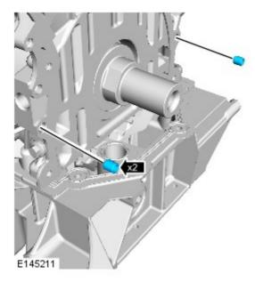
Remove the alignment dowels (if equipped).
