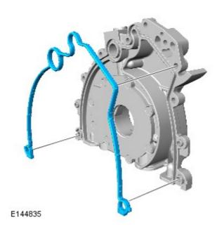
Install a new oil pump gasket.
