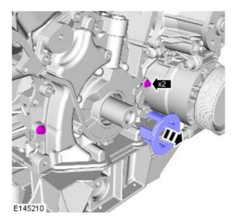
Install two bolts to the oil pump, only finger tighten at this stage.
