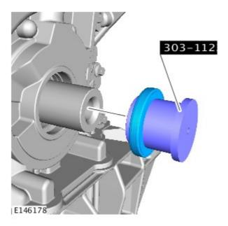
Install the special tool to the crankshaft.
