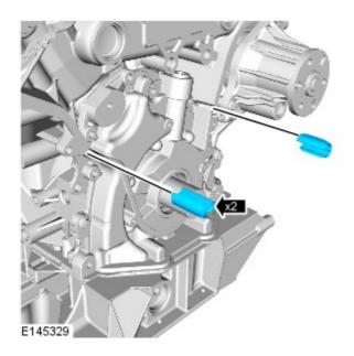
Install the timing belt cover sealing strips.
