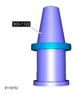
Install a new crankshaft front seal to the special tool.
