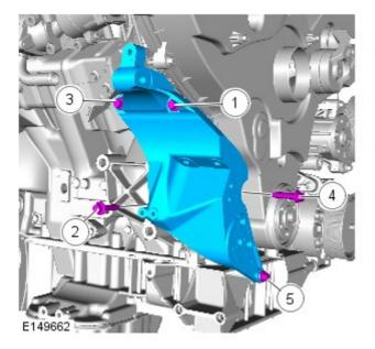
Tighten the bolts in the sequence shown.
