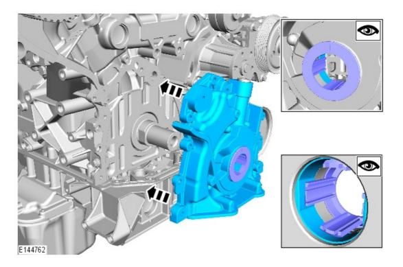
Check the oil pump to engine block alignment.
