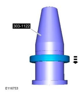
Reposition the crankshaft front seal along the special tool.
