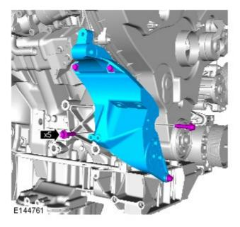
Remove the generator mounting bracket.
