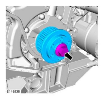
Install the crankshaft pulley.
