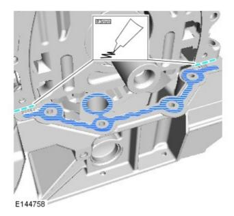
Apply sealant WSE-M4G323-A5 in an 3mm bead to the two areas shown, also apply a smear of sealant to the gasket face as illustrated.
