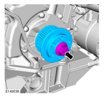
Remove the crankshaft pulley.
