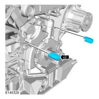
Remove the timing belt cover sealing strips.
