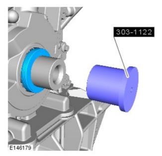
Remove the special tool from the crankshaft.
