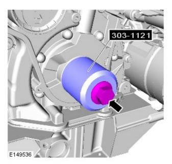
Install the special tool to the crankshaft.
