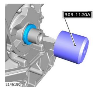
Install the special tool to the crankshaft.
