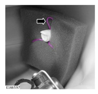
Install the retaining frame onto the smaller foam baffle in the fuel tank.
