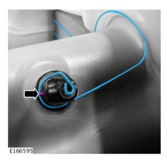
Install the retaining frame onto the tank, as shown in the illustration.
