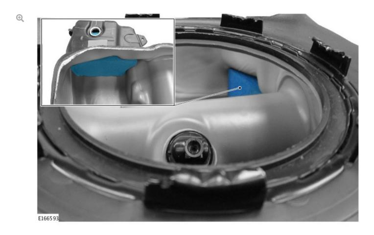
The foam baffle block should now be positioned as shown. If the block is not positioned as shown repeat steps 9 to 13 and inspect again.
