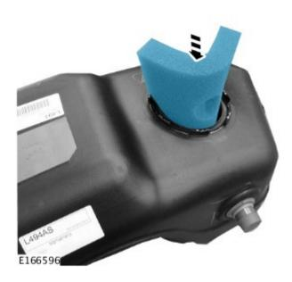
Install the small foam baffle in the active side of the fuel tank.
