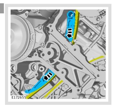
Remove the timing chain guide.
