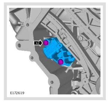
Remove the timing chain tensioner.
