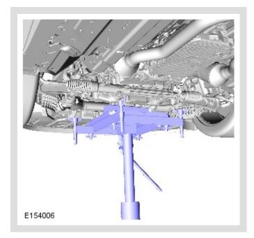
Using a suitable hydraulic jack, support the engine.
