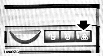
This additional feature may be switched on or off using the forward alert switch as indicated When the indicator lamp in the switch is on, forward alert is active.
