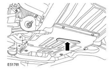
Position the lifting pad of the hydraulic jack in the centre of the recess in the engine undershield.
