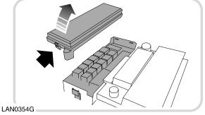
The engine compartment fuse box is located at the rear of the engine bay. To view the fuse box, the under-bonnet cover will have to be removed. See **UNDER-BONNET COVERS**, **218**. The plastic lid of the box is removed by pressing the plastic tabs in.
