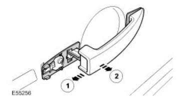
4. To remove the exterior front door handle, after removal of the door trim pad and regulator.
