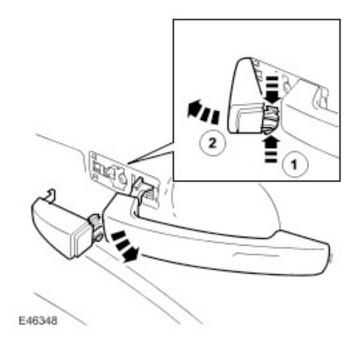
3. To remove the exterior front door handle, without removal of the door trim pad.
