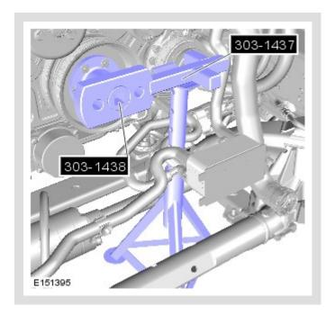
Using a suitable stand, support the special tool.
