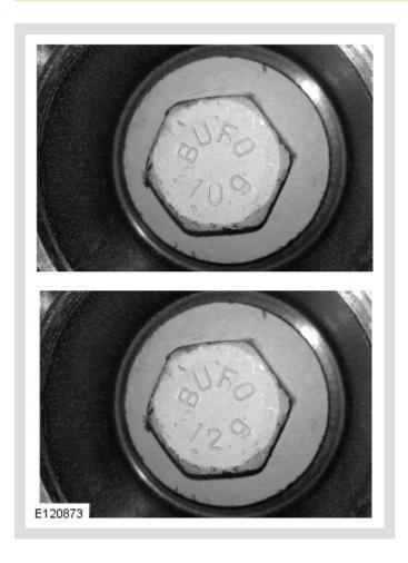
Note the markings on the crankshaft pulley bolt.
