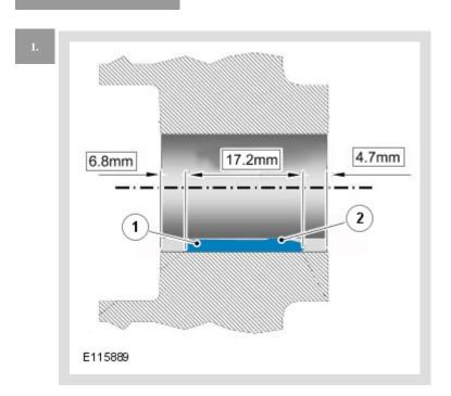
1. Apply RTV sealant to the crankshaft pulley keyway.
