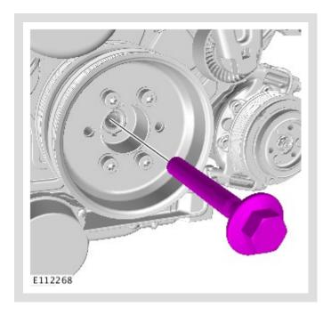
Install a new crankshaft damper bolt.
