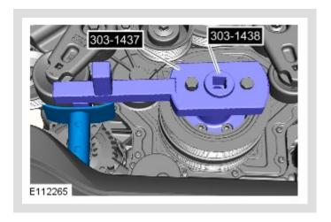
Using a suitable stand, support the special tool.
