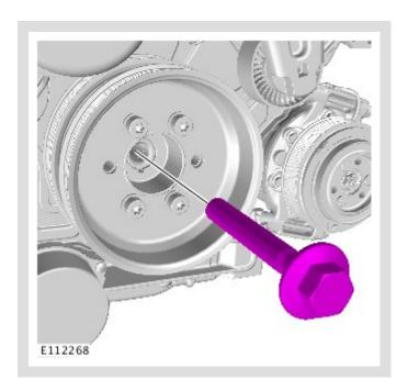
Remove the crankshaft damper bolt.
