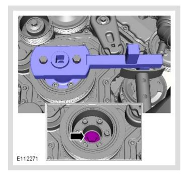
Remove the crankshaft damper bolt, make sure the bolt thread direction has been noted as described in step 8.
