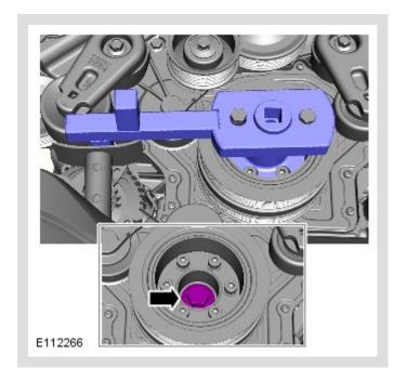
Tighten the crankshaft pulley bolt. Make sure that the socket is turned through 270 degrees not the torque wrench.
