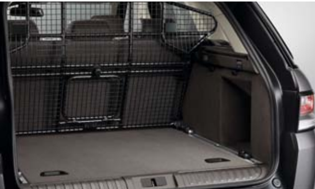
Luggage Divider – Full Height VPLWS0235 The Luggage Divider is designed to prevent cargo from entering the passenger compartment. It incorporates a useful integral ski hatch that allows longer items to be carried where a suitable rear seat option is fitted. Luggage Divider – Half Height VPLWS0236 Luggage Divider – Loadspace Partition* VPLWS0237
