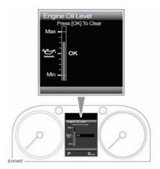
If the oil level is within the required operating range, the message **Engine Oil Level OK** will be displayed. Do not add any additional oil to the engine.
