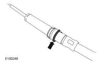
${\bf 3.}$  NOTE: Make sure that the brake cable circlip is positioned as shown.
