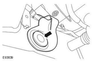
**9.** CAUTION: The fuel tank breather line bracket can be easily damaged when releasing it from the chassis.
