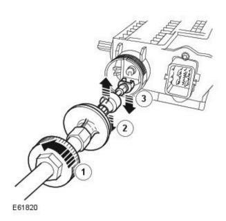
**12.** CAUTION: Make sure that no dirt or moisture enters the actuator during cable replacement.
