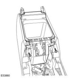
10 . Remove the wiring harness.
