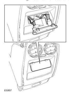
7. Remove the floor console register trim panel.
