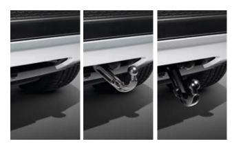
Electrically Deployable Tow Bar VPLWT0111, VPLWT0123, VPLWT0122
