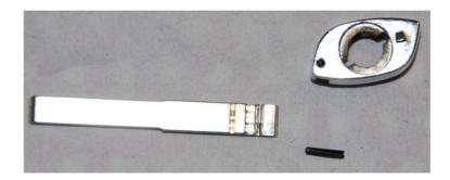
We will use the new blade holder and roll pin with the original key blade.
