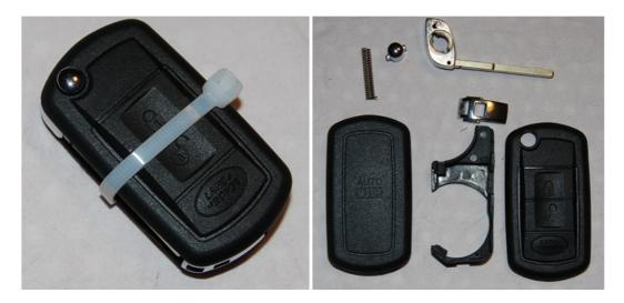
3) Start disassembly of the old key fob. Remove the key blade from the fob by knocking out the roll pin (carefully) with a suitable punch or an old drill bit of the correct size. (This is when you should protect your fingers and eyes in case the punch shatters.) You are then left with the good blade and the old roll-pin.
