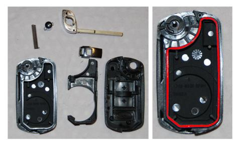
Be careful not to use too much glue but try to run a bead all the way around so to seal the key internals from moisture and dust.
