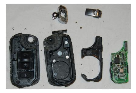
The parts are; front case with buttons, rear case, key blade holder, button and spring, key ring holder, rubber internal board insulator and lastly, the board itself.
