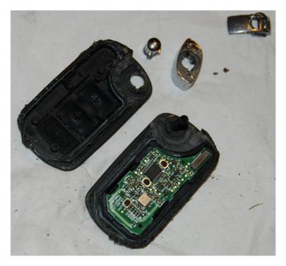
7) Here is an exploded view of all the components from the original key fob:
