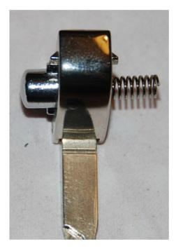
The internal end of the spring goes into the button, the outward pointing end of the spring will locate in the rear case. The button will fit a number of ways into the blade holder but only one way
