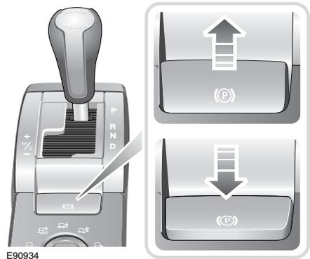
With the vehicle stationary, pull up the lever (arrowed) and release it. The red EPB warning indicator in the instrument pack will illuminate.
