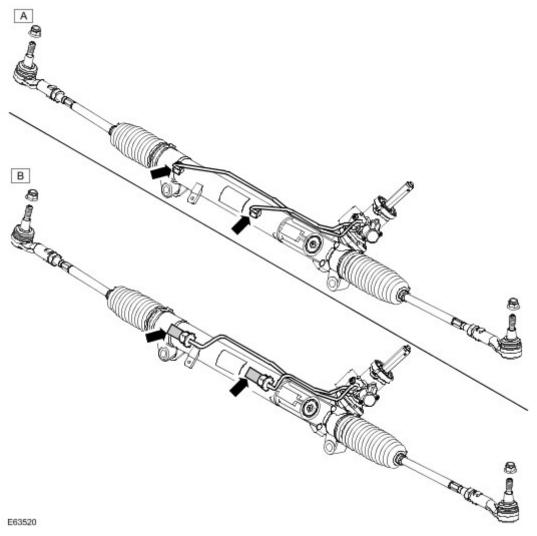
2 . The steering gear can be inspected from the wheelarch area to determine its type.
