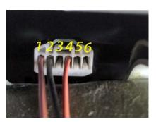
6. Put our control box on hatch panel, secure with provided 3M tape, insert all plugs into control box. Leave power plug as the last one, you will hear a beep once power provided
