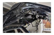
Loosen original gas spring clips by using a screw driver, pull the gas spring out gently. You may need assist to hold the door when removing the original gas spring
