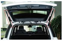
2. Replace original door studs to ours, add our washer under the stud
