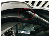
Route strut cable to control box position
