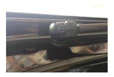
Replace original car body stud to ours, add our washer under the stud
