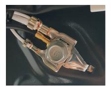
5. Locate lock connector behind original latch, connect our red wire to pin 1, ignore our blue wire
