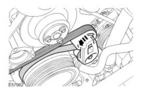
8 . Remove the fluid pump drive pulley.
