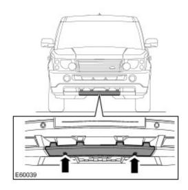
The front towing/lashing eye is accessible after releasing the 2 toggle fasteners securing the towing eye access panel and removing the panel.
