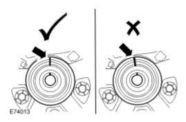
CAUTION: Correct clockspring alignment can be found by viewing a yellow marker through the window situated on the clockspring face. If the marker is not visible, carefully turn the clockspring. If the turning force increases before the marker is visible, reverse the direction to avoid component damage.
