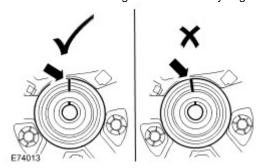
CAUTION: Make sure the wheels are in the straight-ahead position. Failure to follow this instruction may result in damage to the components.
