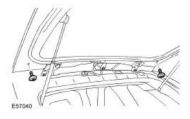
Remove the 3 nuts. Close the liftgate.
