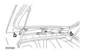
Remove the 2 Torx bolts. Close the liftgate glass.
