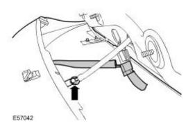
Disconnect the electrical connector. Disconnect the washer jet hose.
