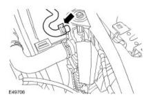
9 . Remove the front RH splash shield.
