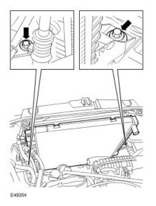
$\ensuremath{\text{24}}$  . Tie the A/C condenser forwards, clear of the radiator.
