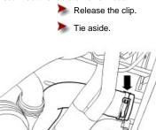
14 . Tie the engine air intake duct towards the engine.
