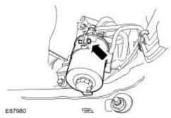
5. Remove the fuel filter bracket. Remove the 2 bolts.
