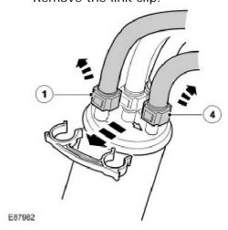
7. Install the link clip to hold lines 1 and 4 together.
