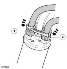
4. Correct connector and line installation shown.
