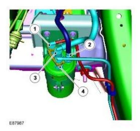
5. Install the fuel filter support bracket.
