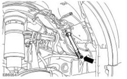
12. **NOTE:** If the knock has been eliminated at step 11, return the vehicle to the customer without refitting the front dampers. It is not necessary to install front body mount dampers on dynamic Response equipped vehicles. If the knock is still evident, carry on from step 13.
