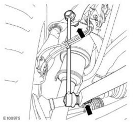
3. Check torque of actuator arm flange bolts to actuator body.
