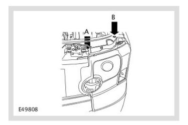
Adjust the headlamps using a suitable tool.
