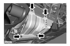
11 . Remove the RH mass air flow (MAF) outlet pipe and connecting tube.
