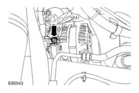
15 . Release the ground cable from the generator.
