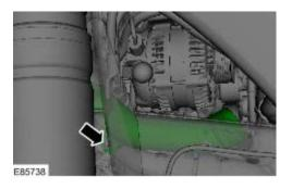
13 . Disconnect the generator electrical connector.
