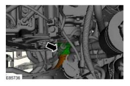
7. Remove the cooling fan shroud.
