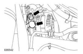
14 . Disconnect the battery positive cable from the generator.
