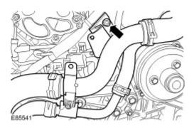
${\bf 6}$  . Release the LH turbocharger intake tube.
