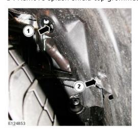
3 . **NOTE:** Front left-hand body mount damper shown with splash shield removed for clarity, right-hand body mount damper similar.
