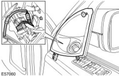
2 . Starting at the lower edge, carefully remove the grab handle cover.
