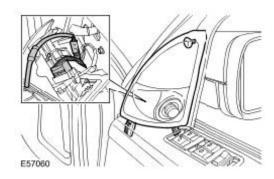
2. Starting at the lower edge, carefully remove the grab handle cover. \*Release the 3 clips.
