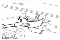
5. Remove the front door trim panel.\*Disconnect the 5 electrical connectors.
