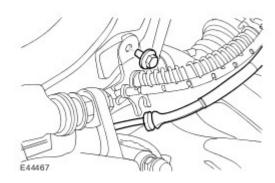
CAUTION: The brake pad wear indicator sensor is easily damaged. Do not use a lever to remove the sensor. Use fingers only.
