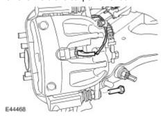
6 . Remove the brake pads.
