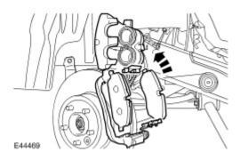
7 . Remove the brake caliper upper bolt.
