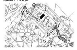
5 . Remove the transmission selector lever mount bracket. Remove the 4 bolts.
