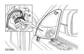
2 . Starting at the lower edge, carefully remove the grab handle cover. Release the 2 clips.
