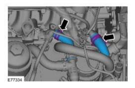
4 . Release the EGR valve inlet tube.Remove the 2 bolts.
