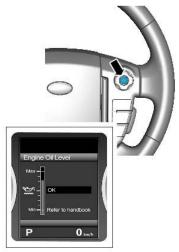
21. Scroll through the trip menu to access the engine oil level display.
