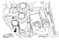
3 . Reposition the coolant expansion tank.
