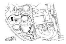
4 . Remove the engine coolant level switch.
