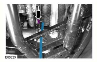
8. Close the radiator drain tap and remove the hose.
