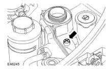
14. Loosen the cylinder head bleed hose bleed screw.
