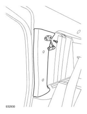
5 . Remove the 2 C-pillar retaining clips.
