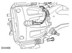
5. Remove the brake pads.
