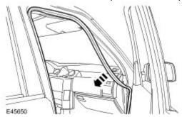
2 . Remove the instrument panel end panel.
