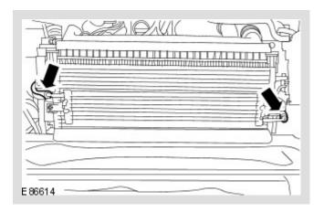
Disconnect the 2 coolant pipes from the auxiliary radiator.
