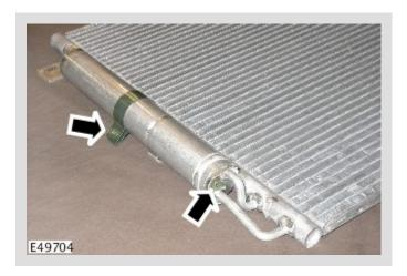
Remove the receiver drier.
