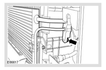
Release the A/C refrigerant lines bracket.
