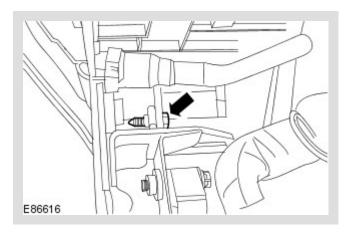
Release the air duct from the cooling module.
