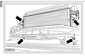
Remove the condenser core.
