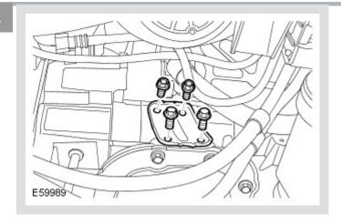
Remove the starter motor support bracket.
