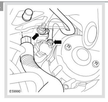
Remove the starter motor.
