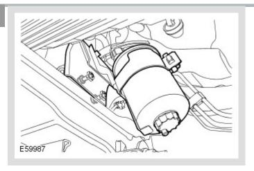
Reposition the fuel cooler and the fuel filter housing and support bracket.
