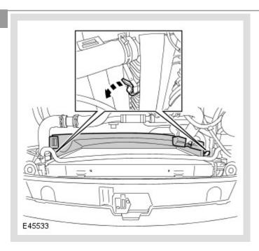
Remove the lower fan shroud.
