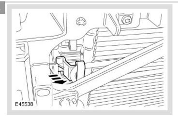
Remove the power steering fluid cooler line clip.
