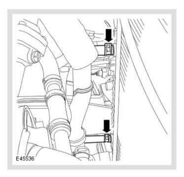
Disconnect the transmission cooler hoses.
